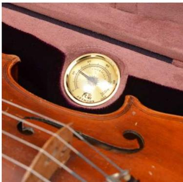
In some cases there have been used a **hygrometer** to measure the humidity. The device is necessary in the case of the luthier instrument made of wood. Air humidity has a significant impact on the technical condition of the instrument, and thus the sound (at too low humidity wood dries up and breaks - instrument loses sound). Best moisture for the luthier instrument is 45-70%.
